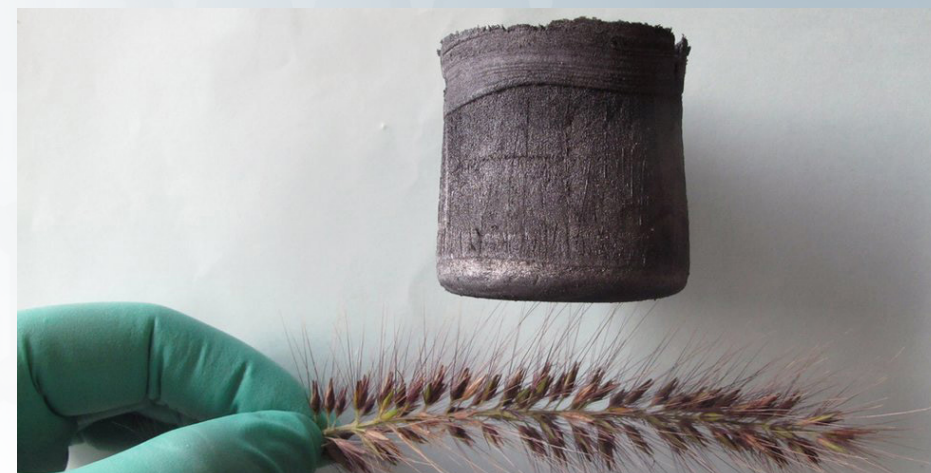
Cilindro de aerogel grafeno de 100 \text{ cm}^3 sobre una espiga de Sun, H., Xu, Z. and Gao, C. (2013), Multifunctional, Ultra-Flyweight, Synergistically Assembled Carbon Aerogels. Adv. Mater., 25: 2554–2560. doi:10.1002/adma.201204576
